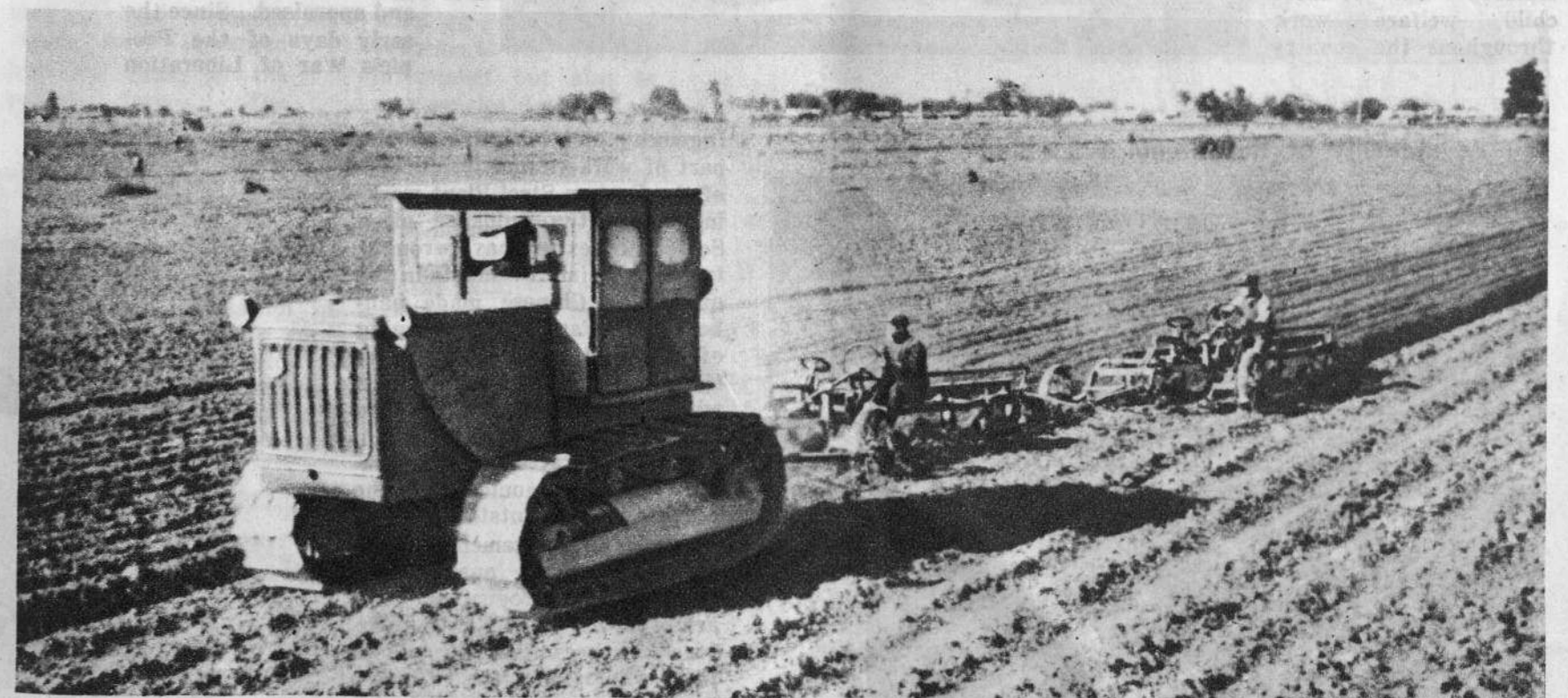
The mighty "No. 80 Stalin" tractor pulls two five-share ploughs, and ploughs from 15 to 20 mou of land in an hour
